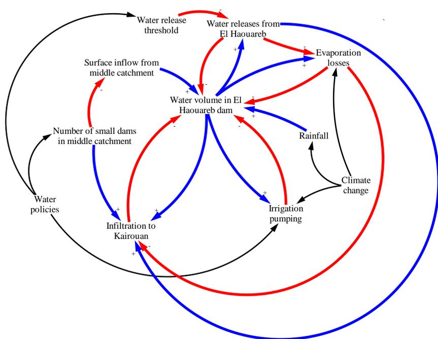
Causal loop diagram showing the feedback relationships between system elements in a sub-model of the Tunisian SDM. Blue arrows represent positive feedbacks, red arrows represent negative feedbacks. Black arrows show external factors that influence system behaviour.
