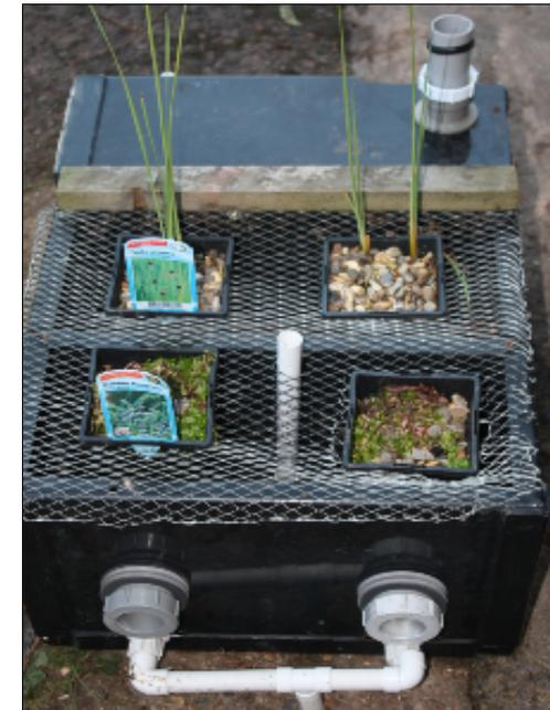
**BabyGROW** is a prototype planted water recycling system for collection & treatment of grey and/or rainwater to improve water quality and provide increased green space
