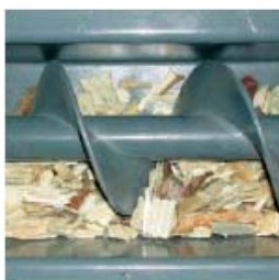
Woodchip transported by an auger screw
