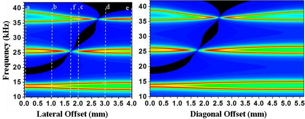
Figure 2: (a) Predicted transmission spectra using a modal matching technique [3], showing the resonant modes of two  $h_m = 12$  mm thick perspex plates separated by  $h_g = 0.94$  mm at increasing lateral plate offsets. Red shading indicates regions of strong transmission, and black indicates transmission amplitudes of less than 0.5%. (b) Similar transmission spectra as (a) with plates offset diagonally.
