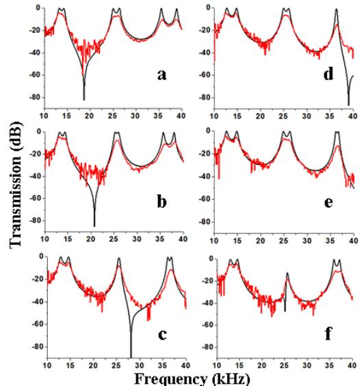
Figure 3: Experimental (red line) and theoretical modelled (black line) transmission results through the ADF structure in air. Graphs (a)-(e) show the transmission for  $h_{\text{off}} = 0$  mm, 1 mm, 2 mm, 3 mm, and 4 mm respectively. Graph (f) shows the transmission for  $h_{\text{off}} = 1.69$  mm.
