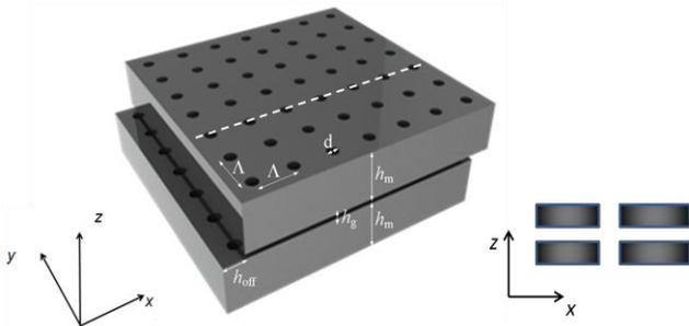
Figure 1: Schematic diagram of ADF structure, with plate thickness  $h_m$ , and gap size  $h_g$ . The circular holes, of diameter  $d$ , are arranged in a square array with pitch  $\lambda$ . The lateral displacement between the plates is  $h_{off}$ . The right-side inset illustrates a cross section of a unit cell (shown with no lateral displacement) taken along the dashed white line.
